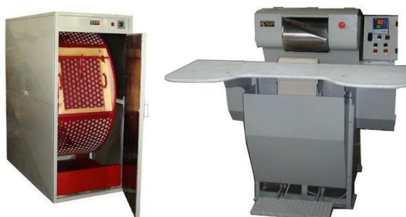
Figure 1 Fur cleaning machines: drum and glazing machine
